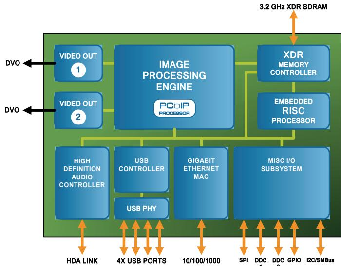
The TERA1100 PC-over-IP (PCoIP) Desktop Portal Engine resides inside a small, simple, stateless access device under any usage scenario. Input comes from the enterprise network via a standard Ethernet connector. Output is driven by a DVI port for video and USB 1.1 ports for peripheral and I/O connections. The net result is a low cost, fan-less, reliable portal-side module that requires minimal IT administration and support since all processing resides on the host PC or workstation.
